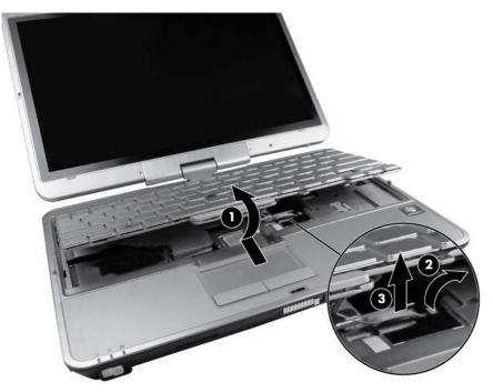
7. Flip the keyboard over to the left and lay it flat (1), then release the ZIF connector that secures the keyboard cable (2) to the system board and remove the keyboard cable (3) from the ZIF connector.
